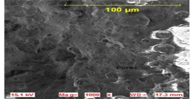
**Figure 4(b). SEM image of 15wt. % GSA Containing Whiteware Body Fired at 1150°C (SP<sub>15</sub>)**
