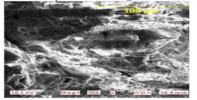
**Figure 4(c). SEM Image of Standard whiteware Body Fired at 1300°C (SP<sub>0</sub>)**
