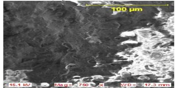
**Figure 4(d). SEM Image of 15wt. % GSA Containing Whiteware Body Fired at 1300°C (SP<sub>15</sub>)**
